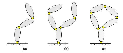
**Figure 1.** Typical topologies of multibody systems. (a) Open-loop topology; (b) Tree topology; (c) Closed chain.
