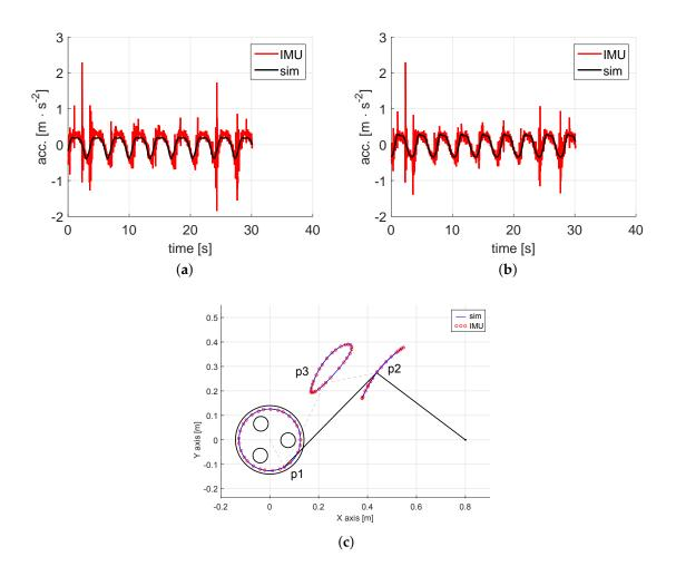
**Figure 6.** More experimental results: (**a**,**b**) acceleration measurements and predictions; (**c**) IMU-based and kinematics-based estimations of each interest point trajectory. (**a**) Acceleration of p3 in *x* axis; (**b**) Acceleration of p3 in *y* axis; (**c**) Trajectory of interest points  $p_1$ ,  $p_2$  and  $p_3$ .
