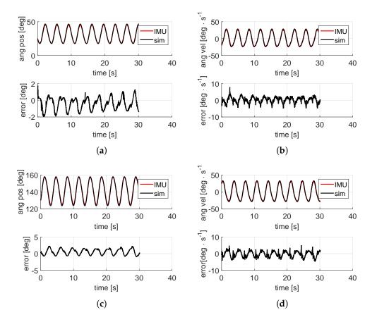
**Figure 5.** Some results from the experimental validation. In all plots, real data from sensors are superposed over the results from kinematics-based estimations. The left-hand figures show the angular positions of the coupler and rocker links and their estimation errors, whereas their corresponding angular velocities are shown in the right-hand plots. (a) Coupler link angular position; (b) Coupler link angular velocity; (c) Rocker link angular position; (d) Rocker link angular velocity.
