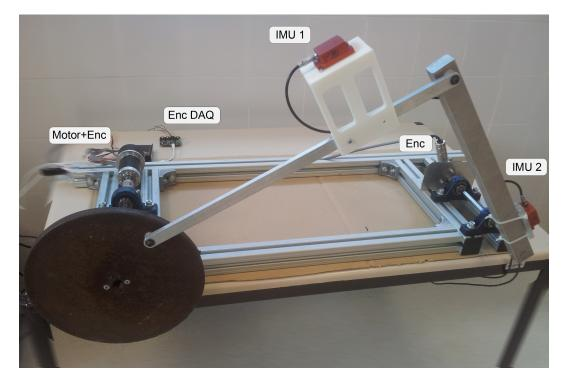
**Figure 4.** Picture of the prototype employed as testbed for the present work. The two inertial measurement unit (IMU) sensors are clearly visible on the top of the coupler link and at the right hand side of the rocker.
