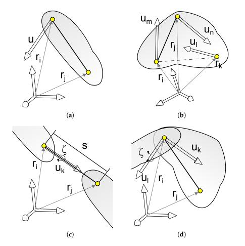
**Figure 2.** Modeling rigid bodies and kinematic constraints under the MBSD approach. (**a**) Two points and a unitary vector; (**b**) An algebraic basis; (**c**) Cylindrical joint; (**d**) Revolute pair.
