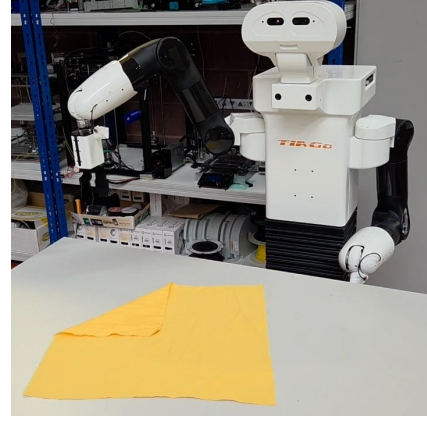
Figure 1: Mobile bi-manipulator robot TIAGo++ in its set up for the folding task.
