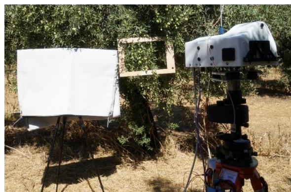
Figure 2: Figure 2: Designed scanning device, consisting of a tripod with a rotating head to enable push-broom operation with the hyperspectral camera.
