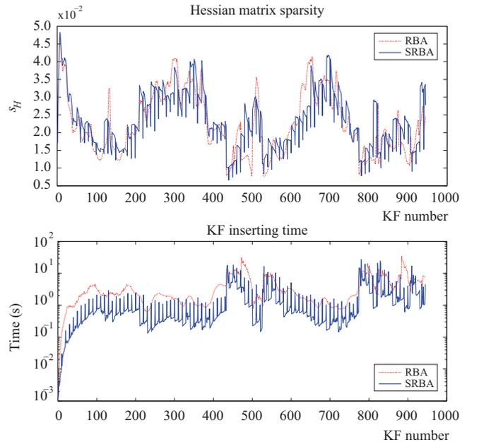
**Figure 13.** Performance comparison for classic (linear) RBA (dashed-red line) and SRBA (solid-blue line). (Top) Hessian matrix sparsity as the ratio of non-zero matrix blocks and (bottom) time spent in optimizing the graph for each KF insertion ( $y$ -axis is logarithmic). In both graphs, smaller is better.
