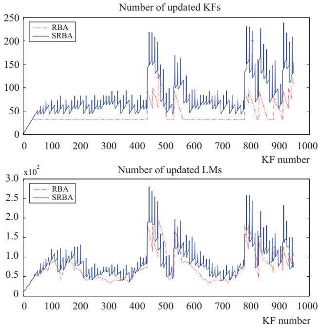
**Figure 14.** Number of (top) keyframes and (bottom) landmarks that are updated at each keyframe insertion (involving graph optimization) for standard RBA (dashed-red line) and SRBA (solid-blue line). In both graphs, larger is better.
