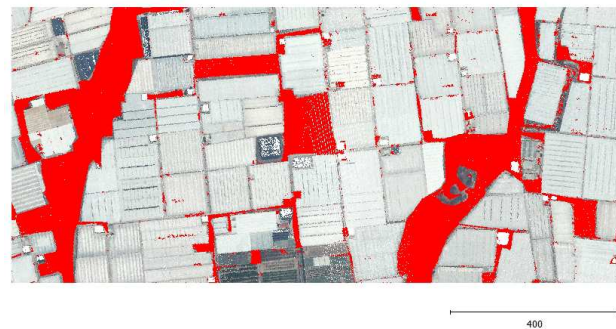
Figure 9. Lidar points (in red colour) automatically classified as "Ground" by applying LAStools software and manual edition
