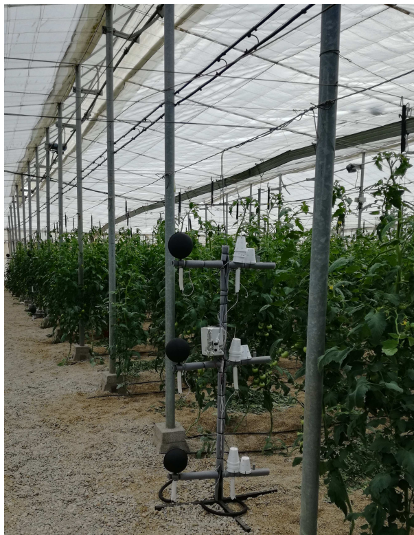
Figure 2: One of the 12 measurement stations located inside the greenhouse.
