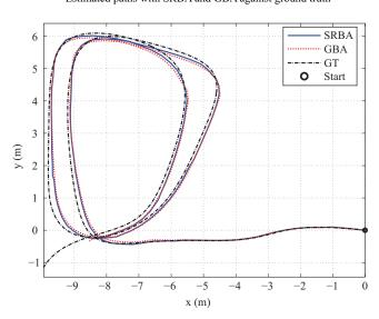
**Figure 10.** Estimated paths for the synthetic dataset with SRBA (blue-solid line) and GBA (red-dashed line). Ground truth is also represented (black dashed-dotted line).
