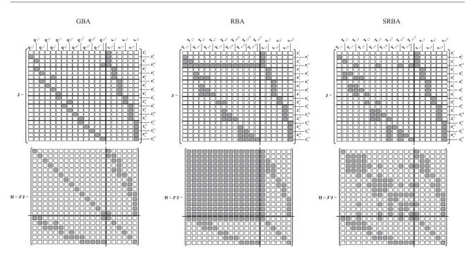
Figure 6. Sparsity pattern of Jacobian and Hessian matrices under the GBA, linear RBA and SRBA approaches for the scenario shown in Fig. 3. Gray squares represent dense blocks within the matrix.
