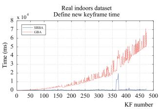
**Figure 15.** Inserting new keyframe time (including graph optimization) comparison for SRBA (blue-solid line) and GBA (red-dashed line) for the real indoors dataset.
