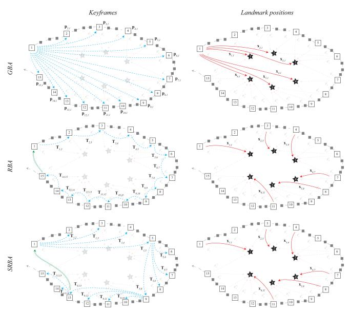
**Figure 4.** Graph representation under a GBA (top), linear RBA (middle) and SRBA (bottom) approaches. Blue-dashed arrows represent edges between KFs and their origins, while red-solid arrows indicate landmark positions with respect to their base KFs. For SRBA, the number of KFs within each submap has been set to 5.
