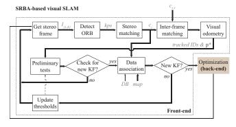
**Figure 1.** Scheme of the proposed SRBA-based visual SLAM system, with the focus on the front-end structure.
