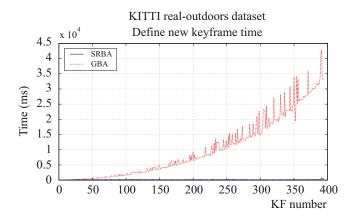
Figure 23. Inserting new keyframe time (including graph optimization) comparison for SRBA (blue-solid line) and GBA
