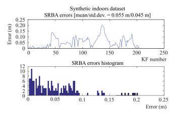
Figure 11. Absolute error and histogram of errors for our SRBA-based method with respect to the ground truth for the synthetic dataset.
