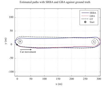
**Figure 19.** Estimated paths for the real outdoors dataset with SRBA (blue-solid line) and GBA (red-dashed line). Ground truth is also represented (black dashed-dotted line).
