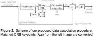
Matched ORB keypoints (*kps*) from the left image are converted into a vocabulary word  $w_i$  employed to query (and which is subsequently inserted into) the image database (DB), retrieving a list of similar images. Then, current left and right keypoints are matched against those from the retrieved similar images by means of the Hamming distance between their descriptors (H blocks). Fundamental matrices **F** are finally employed to discard outliers.
