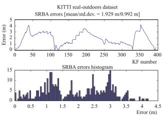
Figure 25. Absolute error and histogram of errors for the SRBA method with respect to the ground truth for the KITTI real outdoors dataset.
