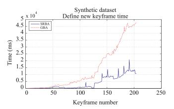
Figure 8. Inserting new keyframe time (including graph optimization) comparison for SRBA (blue-solid line) and GBA (red-dashed line) for the synthetic dataset.
