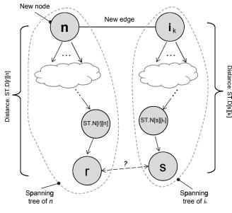
**Figure 5.** Diagram illustrating all the elements considered in the proposed algorithm for incremental update of STs. The creation of a new edge between n and  $i_k$  may become a shortcut that changes the shortest paths between nodes at each side of the new edge.
