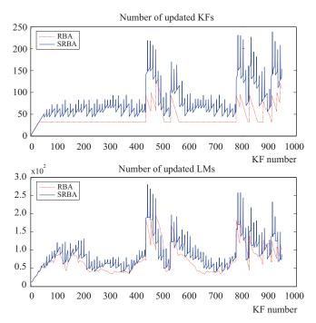
**Figure 14.** Number of (top) keyframes and (bottom) landmarks that are updated at each keyframe insertion (involving graph optimization) for standard RBA (dashed-red line) and SRBA (solid-blue line). In both graphs, larger is better.
