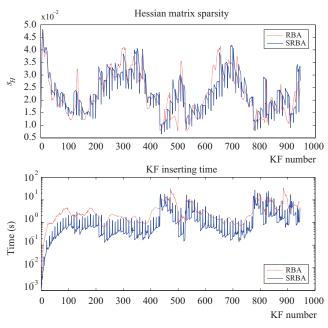
**Figure 13.** Performance comparison for classic (linear) RBA (dashed-red line) and SRBA (solid-blue line). (Top) Hessian matrix sparsity as the ratio of non-zero matrix blocks and (bottom) time spent in optimizing the graph for each KF insertion (*y*-axis is logarithmic). In both graphs, smaller is better.
